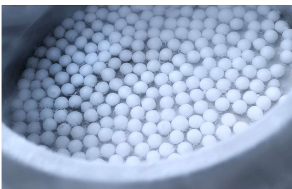
Figure 3: The design uses either a single nozzle or dual nozzles provides the output required per batch. Different size beads could be produced utilising dual nozzles of different sizes. Decontamination priming protocol. Generate up to 4000 beads/hr.
