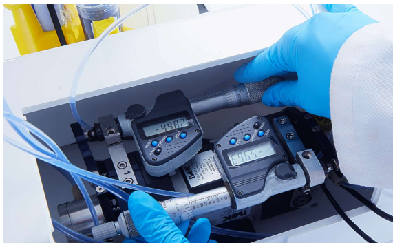
Figure 2: Built in pump and adjustment controls. Volume precision 0.10%
