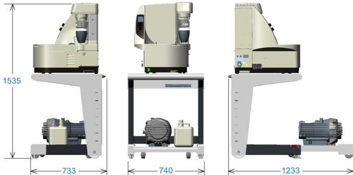
The lower part of the trolley can be partly extended (to 933 mm) to allow access to items on the lower shelf, or fully extended for improved stability when moving.
